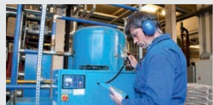
The quantitative leakage measurement determines not only the location of a leak but also the amount of leakage.
