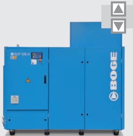
BOGE's frequency controlled SLF machines with a direct drive and frequency controller offer an extremely flexible system that reacts spontaneously to changes in the operator's compressed air demand. If the pressure value changes, the free air delivery is synchronised automatically. A temperature-controlled frequency converter can also be supplied, if required, to adjust the fan output to match the actual demand for cooling air.
