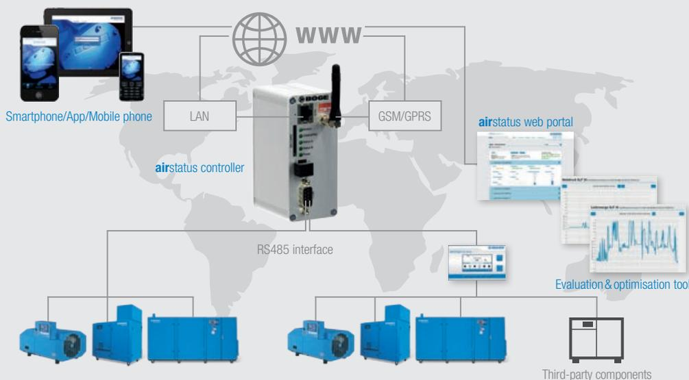
**BOGE airstatus saves and presents you with the process values of your compressed air station, giving you information regarding potential areas of optimisation. You can receive, evaluate and graphically display this data using the BOGE app, for example, or using the airstatus web portal.**
