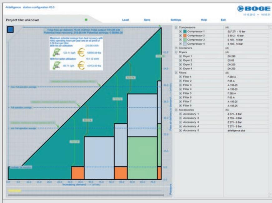
Examining the entire system makes it possible to configure all of the components efficiently. Potential savings can be calculated long before actual production begins.
