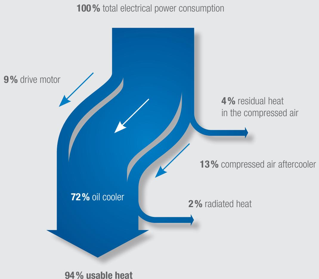
Of the 100 percent of the mechanical energy applied to a screw compressor, an average of 2 percent is lost as heat radiation, while a further 4 percent remains in the compressed air as residual heat.
