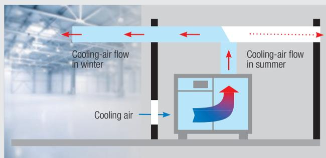
All BOGE screw compressors are sound insulated and equipped with an internal fan. This means that they can be connected to a heating duct system without any problems. Compressors that are not enclosed (e.g. most piston compressors) can be converted for heat recovery by fitting a specially adapted sound hood. In addition, heat exchangers can be installed in the ducts and used to heat process water.
