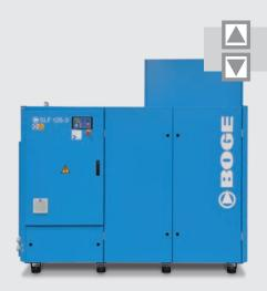
BOGE's frequency controlled SLF machines with a direct drive and frequency controller offer an extremely flexible system that reacts spontaneously to changes in the operator's compressed air demand. If the pressure value changes, the free air delivery is synchronised automatically. A temperature-controlled frequency converter can also be supplied, if required, to adjust the fan output to match the actual demand for cooling air.
