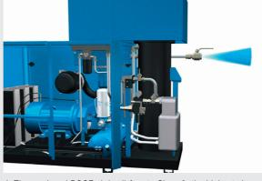
4. The produced BOGE air is oil-free to Class 0, the highest class.
