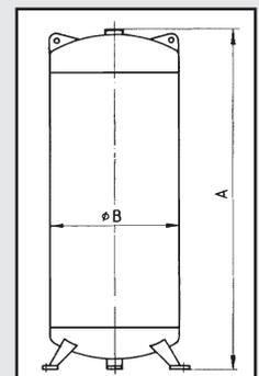
Oxygen receiver manufactured according to directive 97/23/EC, with CE symbol, incl. safety valve and accessories.
