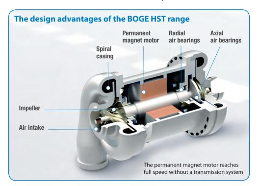
Significantly improved volumetric efficiency:
