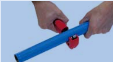
CUTTING Use a tube-cutter to obtain a clean cut.
