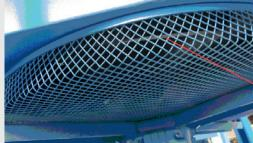
trying to put this wire mesh into CAD made the data volume explode to more than 1000 MByte -> no chance for a CFDcalculation of every detail/wire in reasonable
