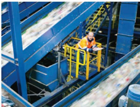
**The conveying speed – three metres per second – is almost impossible for the eye to follow.**
