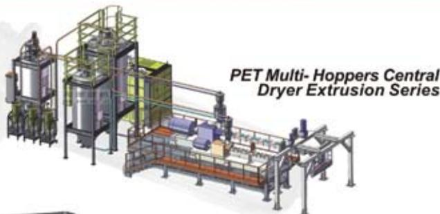
**PET Multi-Hoppers Central Dryer Extrusion Series**
